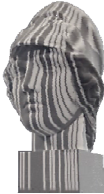
FIG. 3. Shape from structured light
